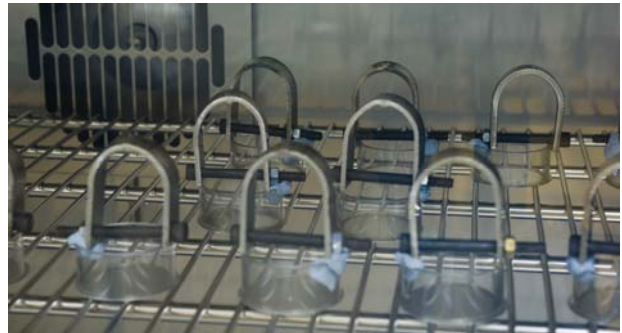
Figure 1 U-Bend samples made from sectioned 316L waste drum material exposed in a humidity cabinet. The outer top surface is stressed to the yield point, and is loaded with salt at different deposition densities by droplet deposition.
