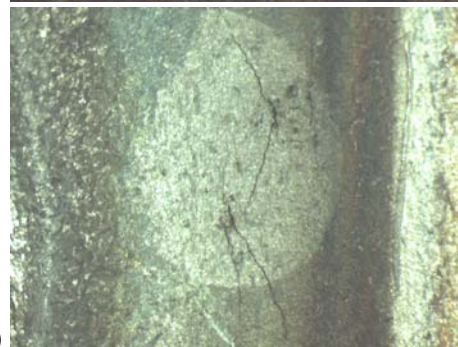
Figure 4 Top surface of 316L U-Bend sample exposed at 40^\circ\text{C} , RH: 30%, 450 \mu\text{g}/\text{cm}^2 deposited from a 5 \mu\text{l} droplet of \text{MgCl}_2 , exposed for 12 months a) before and b) after cleaning.
