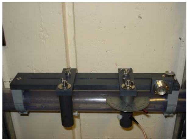
Figure 2 Photograph of the probe holder that was designed and built for this purpose. There are slots for ultrasonic probes to be held at any angle between 0 and 90 degrees.
