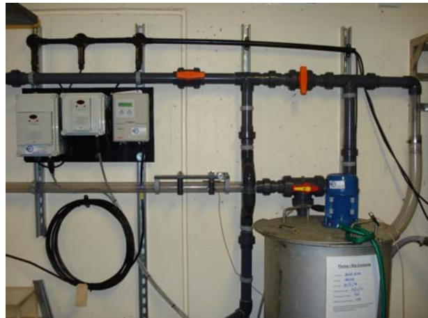
Figure 1 Photograph of part of the new flow loop. Shown: tank, mixer, controls and UDVP probe on test section. Not shown: flow meter and pump.
